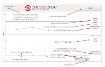
In this mode the software allows the operator to change the calibration and to launch a series of measurements.
