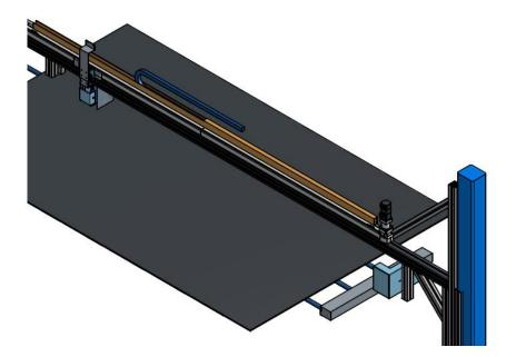
The moving line integration contains a profile structure, for protection the head, measuring an automated axis for the movement of the head, a recalibration and protection electrical box and an cabinet.
