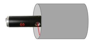
The measuring head with an angle changing tool can be used to measure inside a tube or a pipe. An motorized rotation is also available to automatically measure in all directions.
