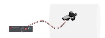
Use the hand-held device to measure different points on the part while linked to the command box
